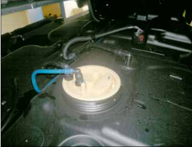
15. Unclip the fuel pipes and sender electrical connection.
