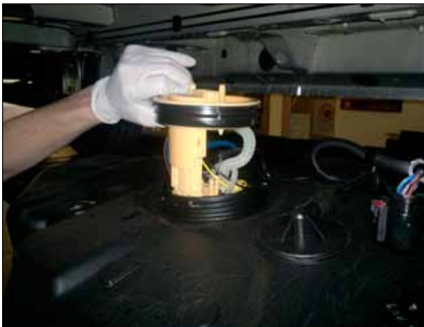
17. Carefully remove sender unit from tank and cover sender hole whilst working on the sender unit to prevent any dirt or debris falling into the fuel tank.
