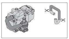
The water pump is fixed to the "fuel connection" side of the heater with rising water inlet connection. The water discharge connection of the water pump faces upwards.
