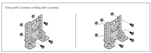
2. Mount special screw M6 x 17 onto the heater.
