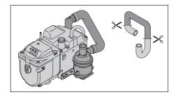
The water pump is fixed to the "water outlet connection" side of the heater with rising water inlet connection. The water discharge connection of the water pump faces upwards.
