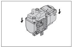
Use 2 hexagon screws M6 x 12 (with adhesive coating) to fix heater to the bracket (tightening torque 6+2 Nm).
