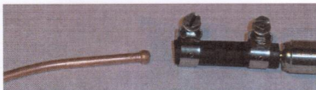
Flared end of copper pipe
