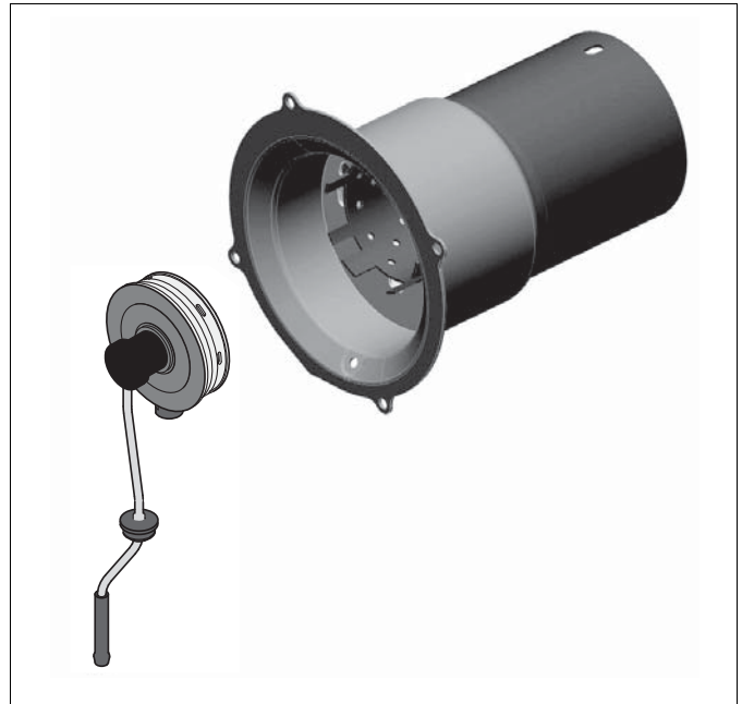
Fig. 206 Evaporator mount (petrol) and combustion pipe
