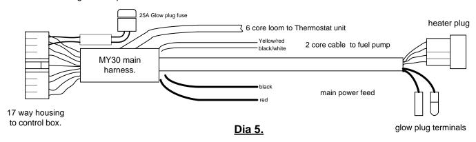
Mount the control box on a flat vertical surface with the 17 way housing at the bottom. Secure in place using the  $4 \times 3/4$ " No10 self tappers provided. Now plug the main harness into the control box and then the heater and glow plug terminals ensuring that they are a tight fit. Plug the 2 core fuel pump loom into the main harness, trim to length, attach the 2 bullet receptacles and plug into the fuel pump - polarity is not important.
