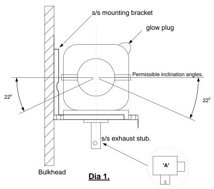
The heater is supplied with a stainless steel 'L' shaped mounting bracket which is designed to be fitted on a vertical bulkhead with the heater sat in it (see dia 1.)The heater has to be mounted in this way for correct operation.
