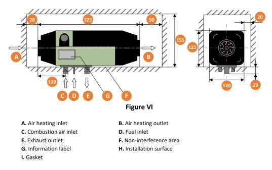
Choose a flat installation surface, any undulations could cause the case to twist and will not ensure an even mount. Make sure there are no foreign bodies between the bottom of the heater and the installation surface itself. This will ensure a good seal between the two. File down any drill holes to again ensure an even mounting surface. Tighten the M6 bolts provided to a torque setting of 6Nm+1Nm.
