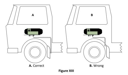
Only use the inlet pipe and exhaust provided with the kit for installation. The exhaust pipe is made of corrugated stainless steel while the combustion pipe is aluminium covered in paper and plastic. **Do not** confuse the two. Use the supplied clamps to fix them securely to the combustion air inlet and the exhaust outlet on the heater. The protective end cap on the outlet of the
