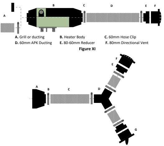
**A.** Heater Outlet **B.** 60mm Hose Clip **C.** 60mm APK Ducting **D.** 60mm 'Y' Branch **E.** 80-60mm Reducer **F.** 80mm Directional Vent **G.** 80mm Open/Close Vent
